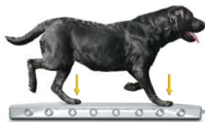
Biomechanical force platform with integrated balance. Speed between 1.7 an 2.1 m/s
